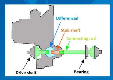
Stub shafts are an unique development of VAG which can be found mainly in Transporter and Van applications.
